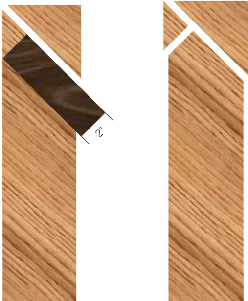
Raker return cut (This must be done to all raker cuts outlined in this section)
