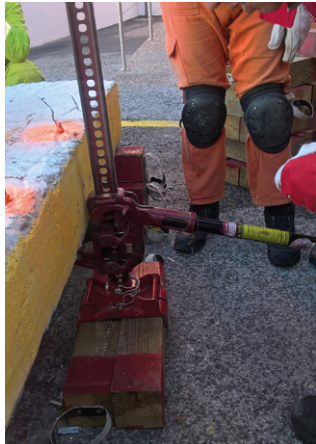
Hi-Lift Jack : used to lift weights up to 2000 kg
