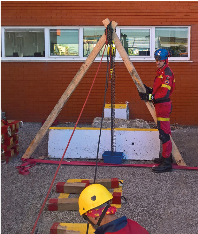
A-frames provide high anchor points for mechanical advantage systems
