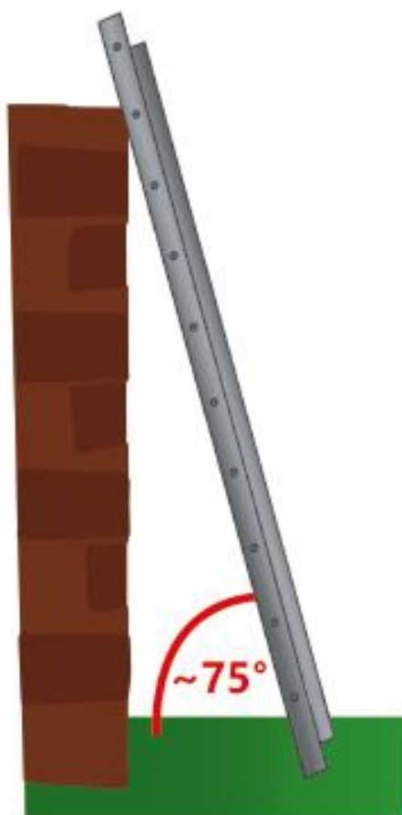
Figure 26: Safe ladder angle
